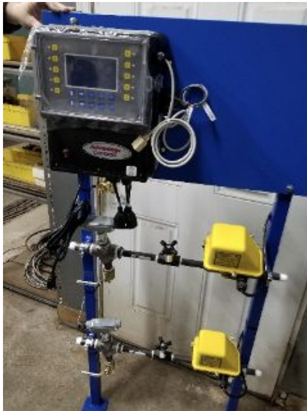
Figure 1 – Automated Surface Blowdown Valve Stand
